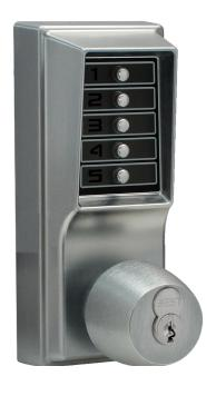
The Simplex 1000 Series provides exterior access by combination, while allowing free egress. This mechanical knob operated lock has a single access combination and is programmed via the keypad without removing the lock from the door. The lock is available in a variety of architectural finishes.
